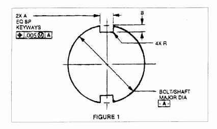
2.1 Prepare key-ways using dimensions noted in Table I and corresponding detail of Figure I.
